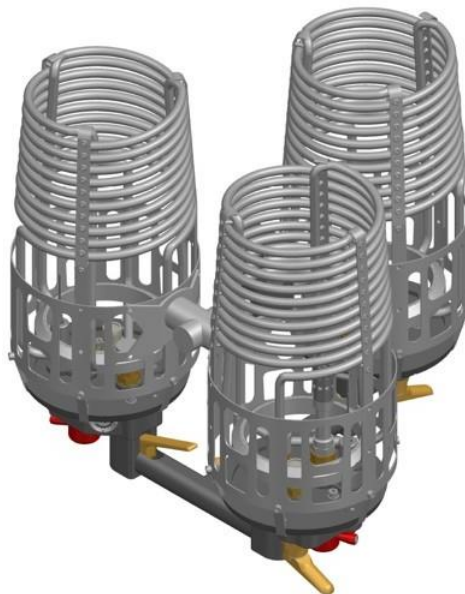
Figure 44. Triple burner general view
