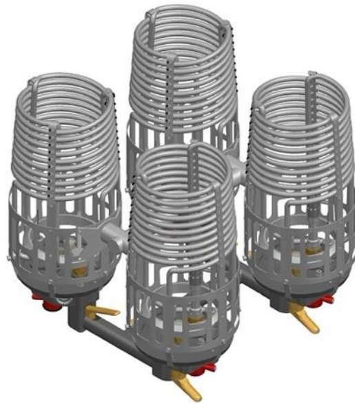
Figure 55. Quadruple burner general view
