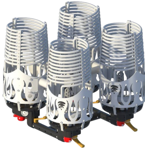
Figure 7. Quadruple burner general view
