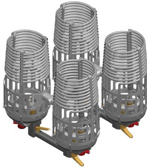
Figure 5. Quadruple burner general view
